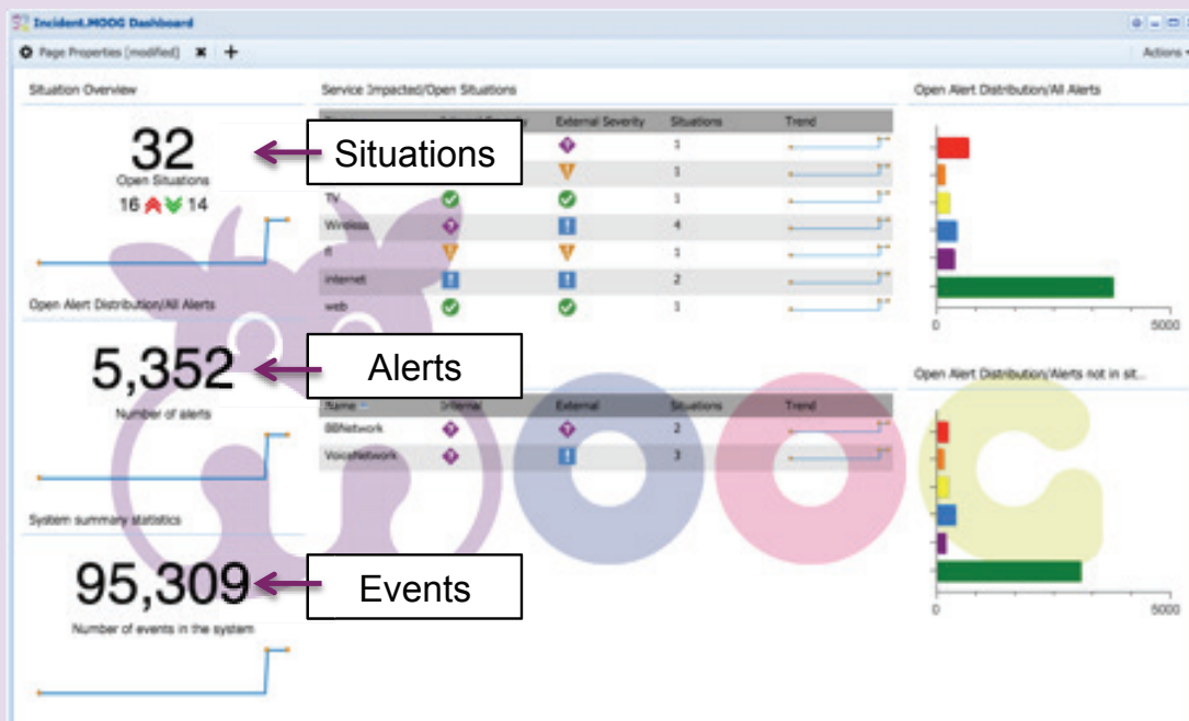
FIGURE 1. Incident.MOOG reduces actionable work items by more than 80%, clustering clusters events across silos to create meaningful Situations with history and context.
